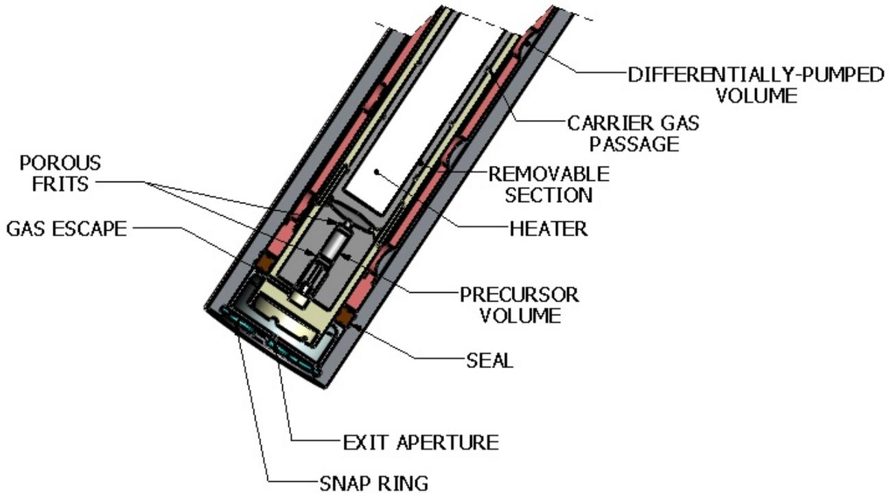
The OMP Doser is supplied with several EXIT APERTURES of various sizes. To exchange or replace the EXIT APERTURE, simply remove the SNAP RING.
